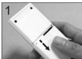
1. Turn off the meter by pressing the “M” button and hold for 2 seconds before replacing the batteries. Slide down the battery cover on the back of the meter by pushing the cover in the direction of the arrow and put the cover aside.
