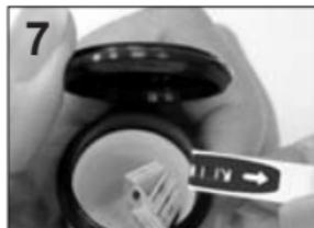
8. Insert a test strip into the meter while the meter is off. The meter will turn on automatically, and you will hear: **“Hello, the Meter is ready.”** A blinking blood icon will be displayed on the screen. You will hear **“Apply blood now.”** If no action is taken in 2 minutes, the meter will turn off automatically. You will hear: **“Goodbye.”**
